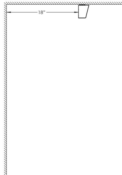
Fixture must be installed at a distance from the wall of 12-18" (recommended 18").
