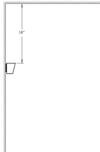
Fixture must be installed at a distance from the ceiling of 12-18" (recommended 18").
